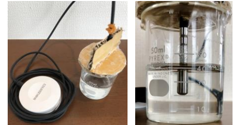
Figure 2: The device to measure the temperature of the central part of liquid
